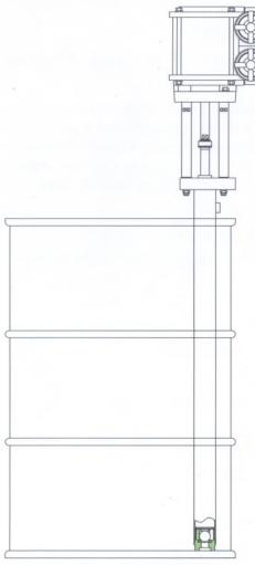
suitable for transferring, Spraying of Lubricating, Rust Proof, Undercoating Fluids (oil, Grease, Wax, Glue etc.)
